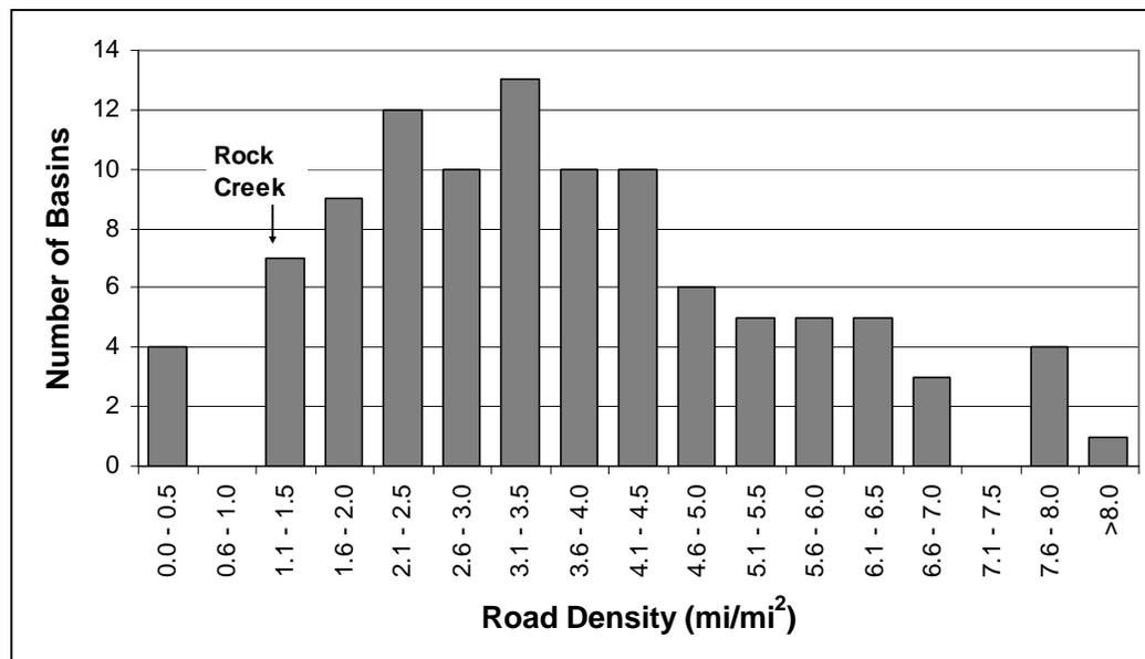
**Figure 5-4. Road Density in Basins on the Eastside of Washington State.** Data compiled from watershed analyses completed under the Washington Department of Natural Resources' Watershed Analysis Methodology. The road density in Rock Creek basin is 1.5 miles per square mile.
